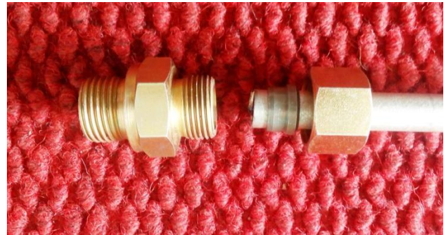
Figure 3.2: Male Stud Connectors.
